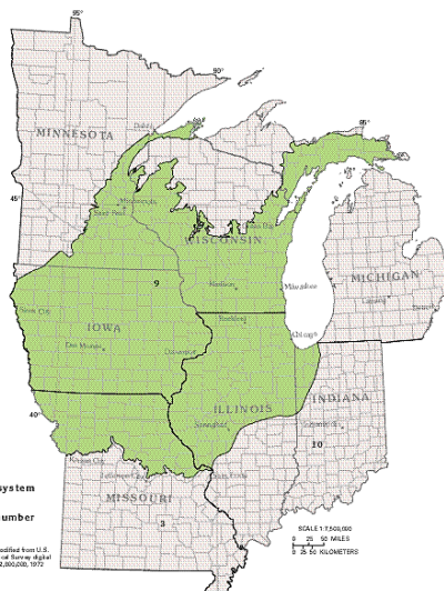
Figure 20. The Cambrian-Ordovician aquifer system, which consists of predominantly sandstone aquifers separated by poorly permeable confining units, extends over a large part of the north-central United States.
